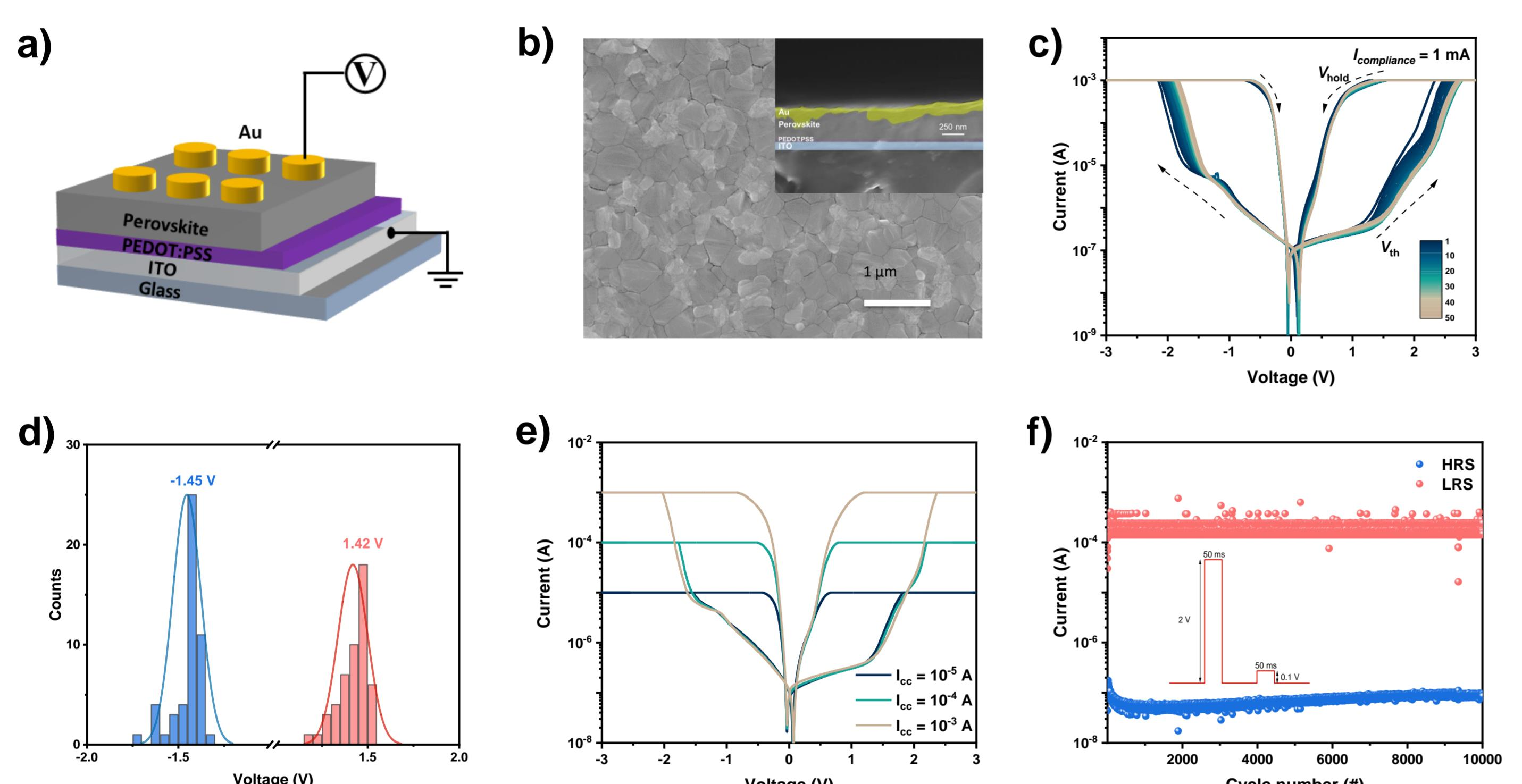
➤ (a) Schematics of biological nociceptor and an artificial nociceptor electrical circuit. (b-d) Threshold, no adaptation, relaxation and (e-g)sensitization characteristics of the perovskite-based artificial nociceptor
