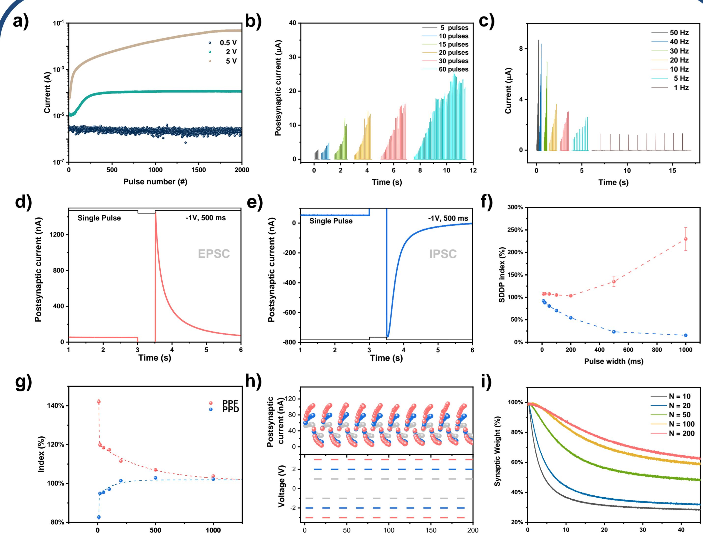
➤ a-c Response current of the perovskite diffusive memristor upon varying voltage pulses number, amplitude, and frequency.
